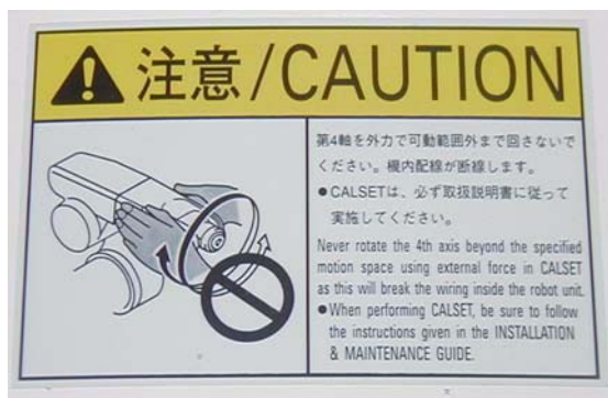
Figure 5-3. Caution Label on Joint 4 Rotation
