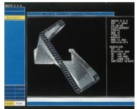
Deformation of competitor's base structure under the same amount of force.
