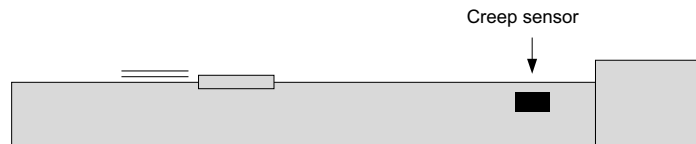
A sensor is provided before the mechanical end and once this sensor actuates, the speed is reduced to perform normal home return operation.
