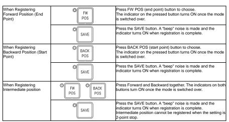
(Note 1) When registering the position with using Jog/Inching Mode, press either Forward or Backward button and hold it down, and the operation mode changes in the order stated below;
