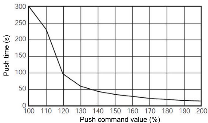
Condition [2] Thrust for continuous operation
