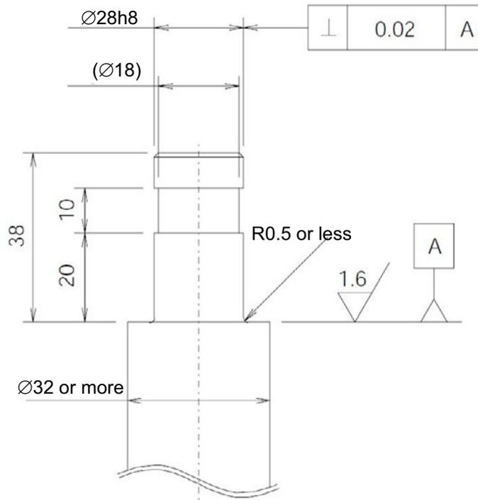
Dimensions of the load cell side where a jig is to be attached
