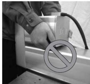
Do not hold the motor cover when transporting the actuator.
