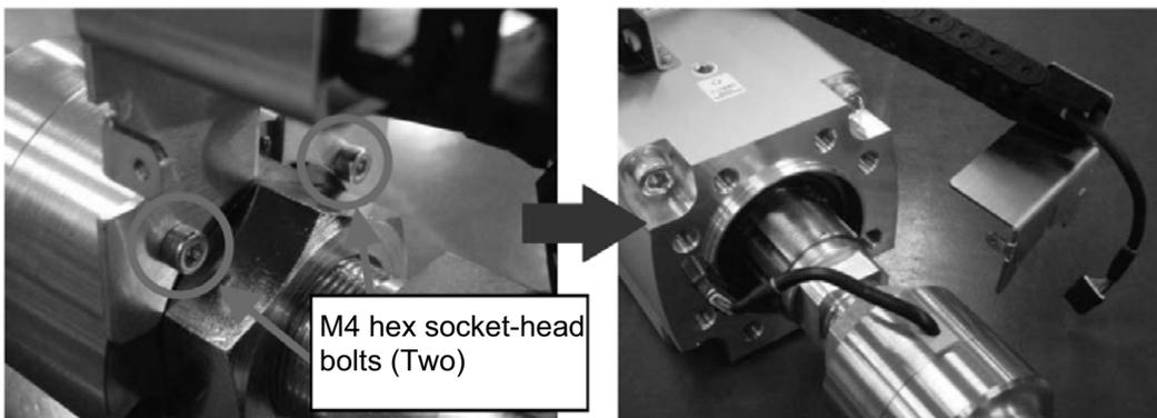
[4] Attach the cable track based on the procedure on the previous page in the reverse order.
