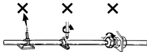
6. Do not pinch, drop a heavy object onto or cut the cable.
