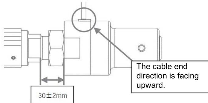
**Caution:** There is an electronic circuit board mounted in the loadcell unit, which is the precision instrument. Handle it with a special care and screw it in slowly. Screwing it in forcefully may cause damage on the electronic circuit board.
