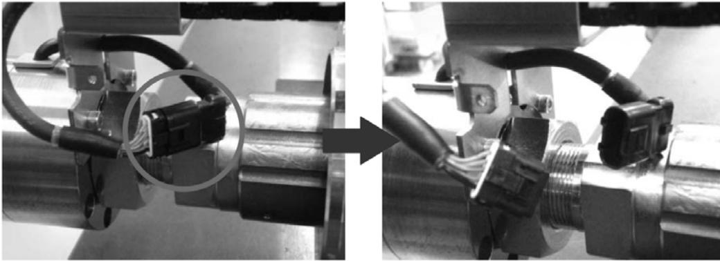
[3] Remove the M4 hex socket-head bolts and remove the cable track from the load cell.
