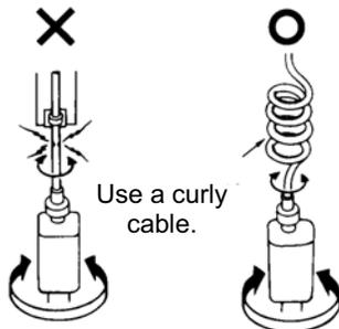
5. When fixing the cable, provide a moderate slack and do not tension it too tight.
