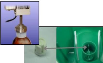
**Capping of Bottles:** Cap rotates to engage slot. Detect and report no/obstructed nozzle. SMAC actuators can adjust force and torque, show the different quality check capabilities such as cap height, torque limit, force required to press in, and even check the clicks on child proof caps.
