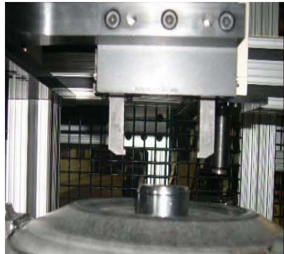
SMAC Gripper featuring 2 independent axis of "finger" control
