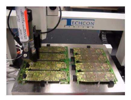
**OVERVIEW:** This application is to dispense dots of solder paste on PCB
