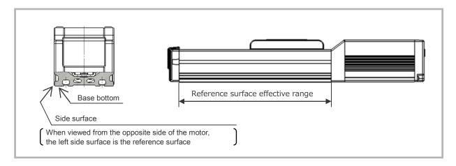
When mounting using the side reference surface, machine the installation surface according to the figure below.
