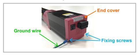
Use a tester to measure the continuity between the fixing screws and grounding surface to check whether it is grounded or not.
