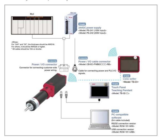
Supply 24VDC to the ELECYLINDER and input a signal from a master device to the ELECYLINDER.
