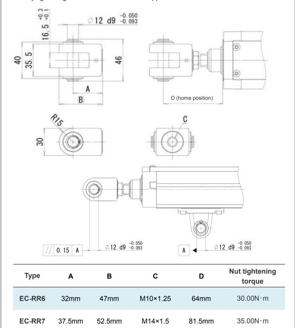
•Body clevis (-QR) mounting method and component dimensions
