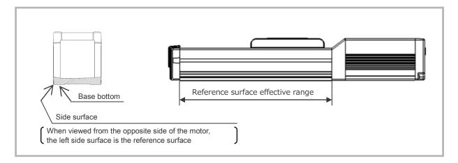
When mounting using the side reference surface, machine the installation surface according to the figure below.
