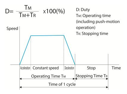
The duty ratio for the ELECYLINDER is limited to the values below.
