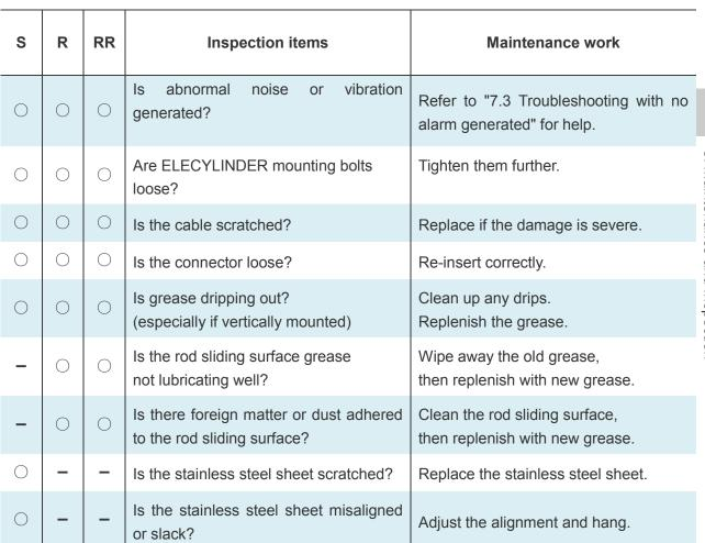
Refer to "8.6 How to replace components" for detailed information about specific component replacement and adjustment methods.
