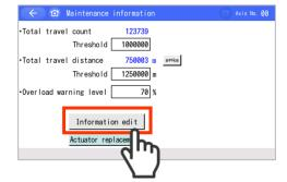
If the actuator has been replaced, touch the "Actuator replacement" button.
