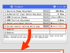
Enable = optimized current for the actual load stops the motor (power saving stop)
