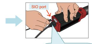
Insert the round connector with arrow mark downward
