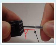
After fully inserting the wire, pull out the precision screwdriver.
