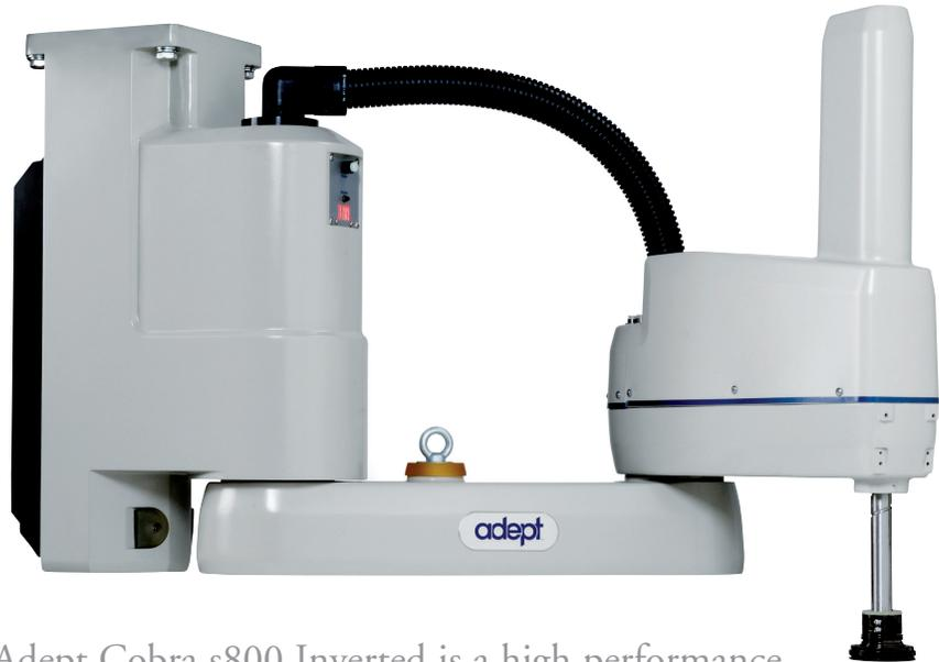
The Adept Cobra s800 Inverted is a high performance robot system designed for packaging and material handling applications. The overhead mounting makes it ideal for mounting above a conveyor belt and minimizing the machine footprint. With an 800 mm reach and 5.5 kg payload this robot is well suited for a much wider range of applications than specialized picking robots.
