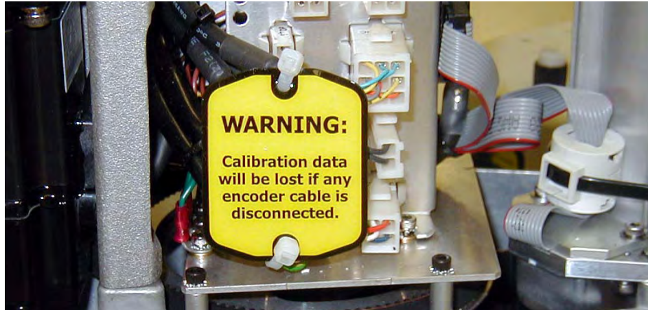
Figure 2-3. Warning Label on Encoder Cables
