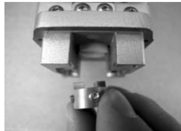
Inserting the coupling (with screws)
