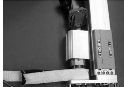
Motor-unit affixing bolts (Use an Allen wrench of 2.5 mm across flats.)
