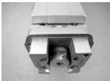
Inserted coupling (with screws)
