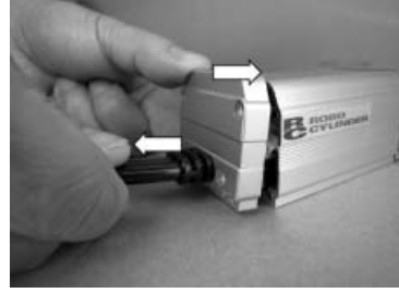
Pull out the cable end while pushing in the motor-end cap.
