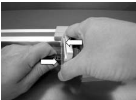
Push in the cable end while pulling out the motor-end cap.
