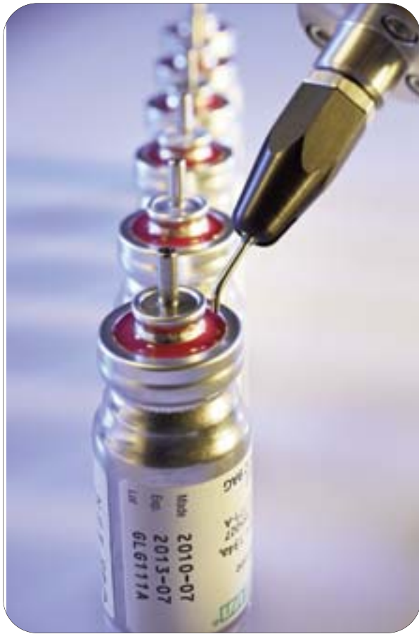
TS5440 - dispensing medical device adhesive
