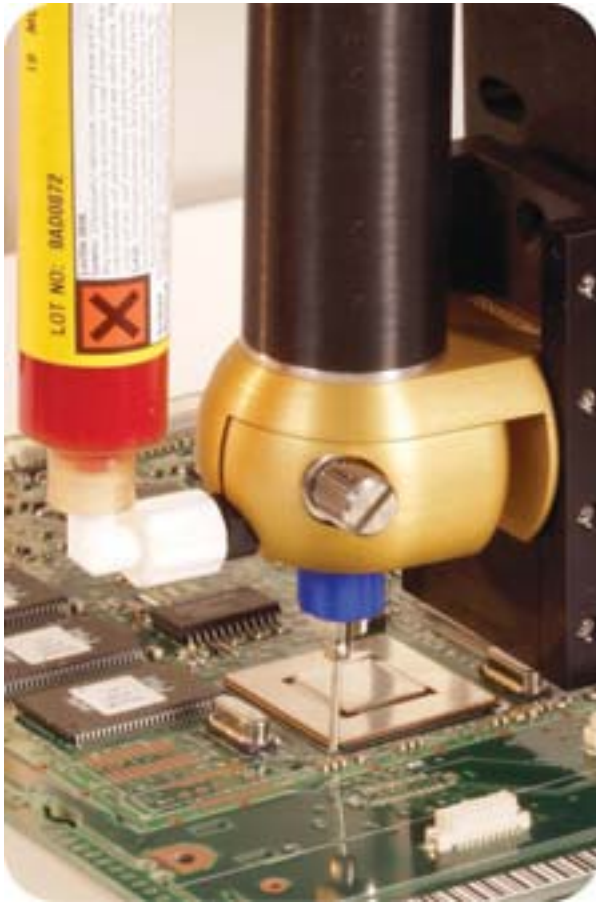
TS5000DMP - performing underfill.
