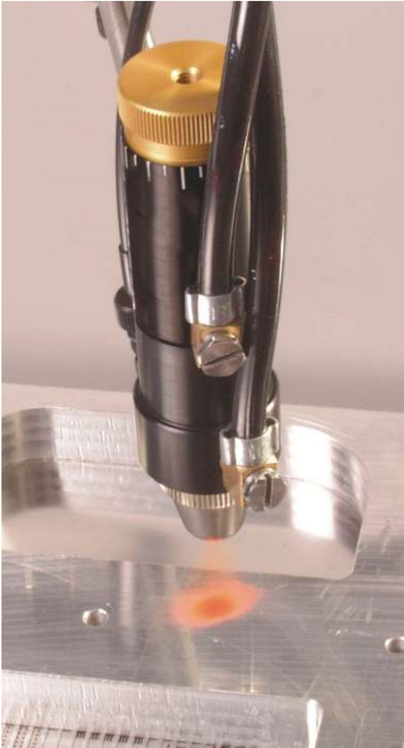
▲ TS5520 - spray marking on metal work.
