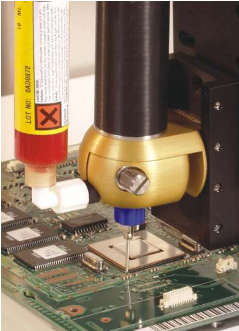
▲ TS5000DMP - performing underfill.
