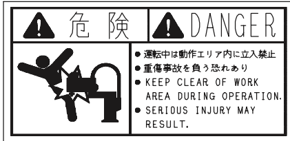
Prohibition of entry into the operation area
